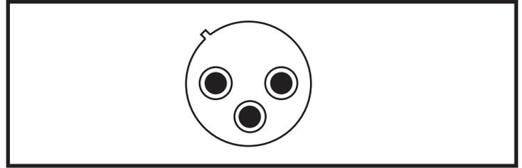
Figure 4. 3-pin Off-Board Charger Socket
