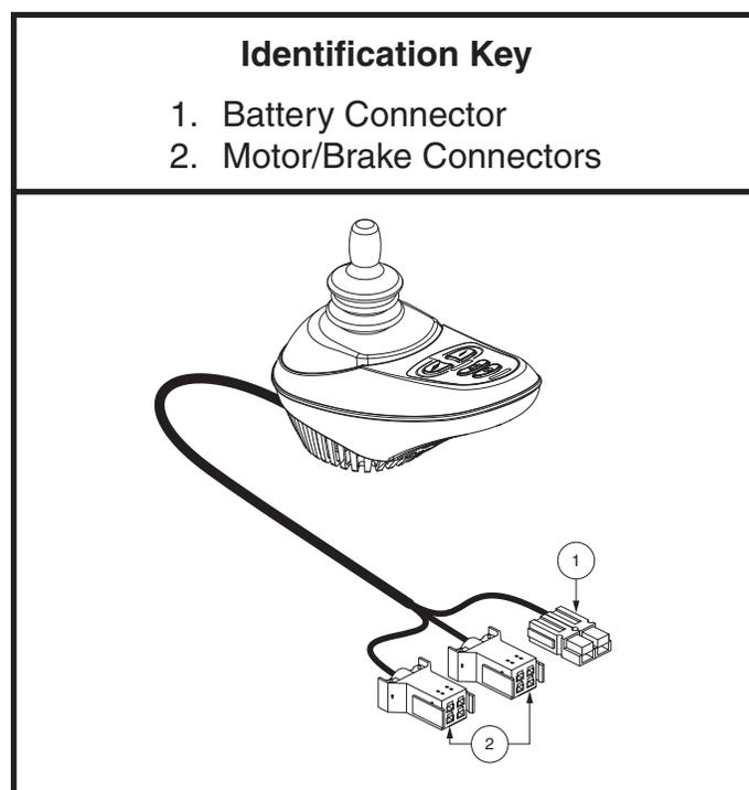
**Figure 2. newVSI Controller (Battery and Motor/Brake Connectors)**
